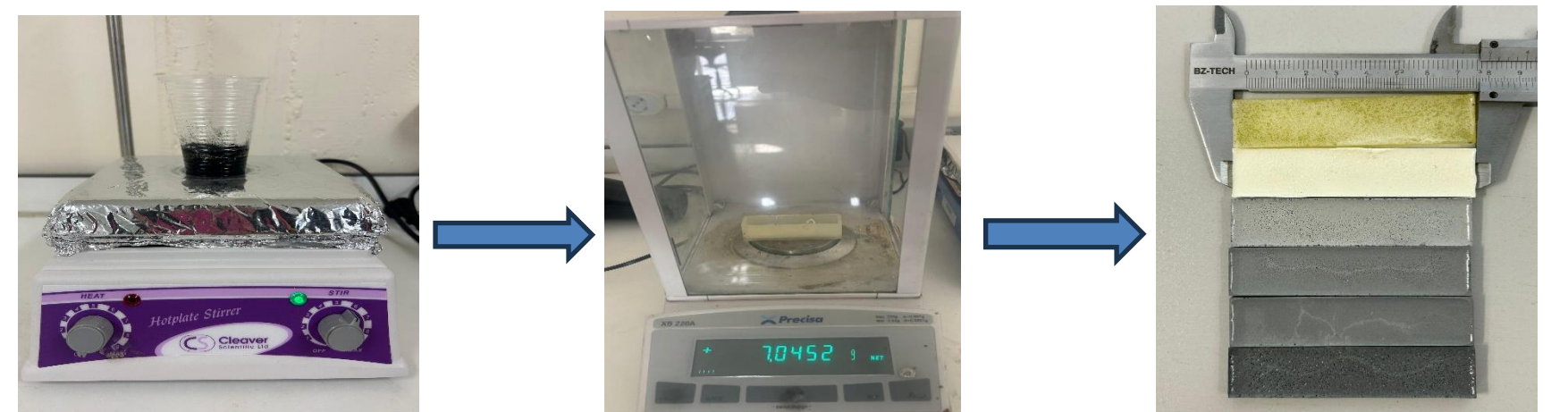
Figure 1. The procedure for producing TiO 2 /CNT reinforced epoxy polymer composites
