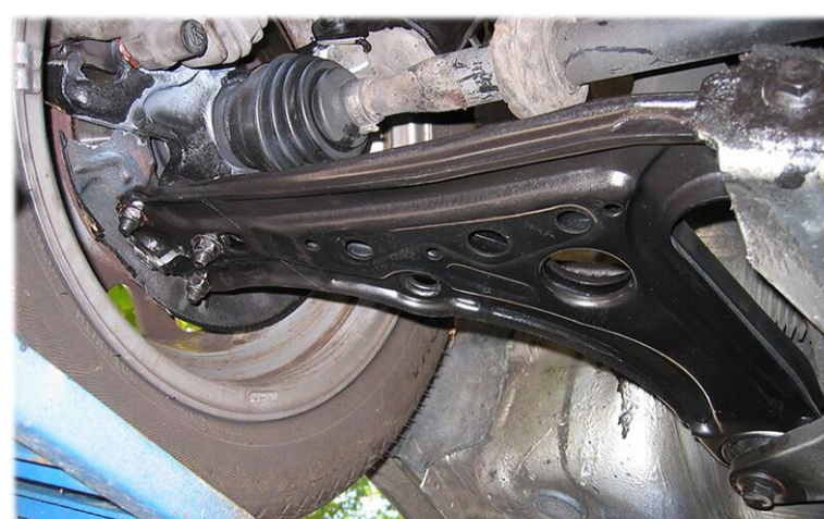
Figure 2. Lower Wishbone Integrated into the Vehicle Suspension System.
